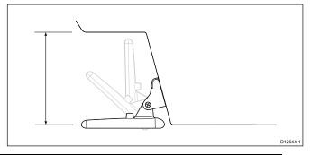
**Note:** Optimum transducer location will vary depending on vessel type. Optimum transducer height and angle should be obtained by testing the transducer with the vessel in the water before locking the transducer's position.
