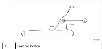
11. Adjust the angle of the transducer using the ratchet mechanism, one click at a time until the transducer face is parallel with the waterline.
