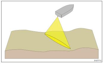
DownVision<sup>TM</sup> is effective at lower vessel speeds. In deeper waters the CHIRP bandwidth is automatically optimized to improve bottom lock and the detection of moving objects (e.g. fish) in the wider water column.
