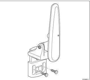
8. Using the screws provided, temporarily secure the mounting bracket using the adjustment slots on the back plate.
