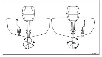
• On a twin engine vessel the transducer should be mounted between the engines.
