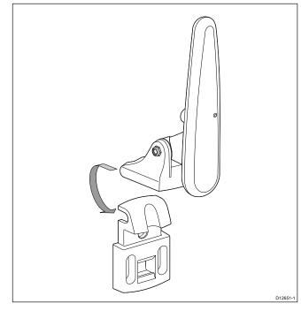
7. Lift up the transducer and pivot arm to access the mounting holes.
