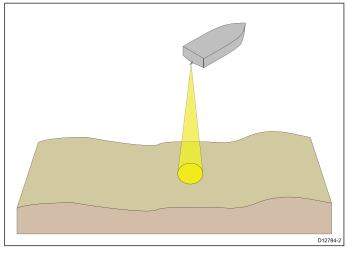
Sonar is effective at a range of speeds. In deeper waters the CHIRP bandwidth is automatically optimized to improve bottom lock and the detection of moving objects (e.g. fish) in the wider water column.
