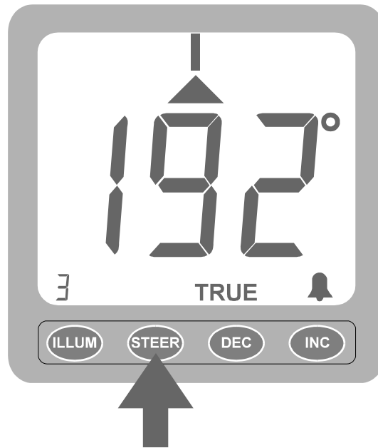
FIGURE 5 - Vessel heading aligned with setting
