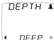
The water depth has increased above or fallen below the preset alarm level.
