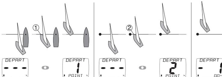
**Note:** The line for Depart calculations is between the positions you set. Set your points as close to the ends of the actual start line as possible.
