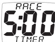
The most convenient way to operate the race timer is to use the Timer Page of the Remote Display. Once started the countdown is available on all displays. See the Remote Display user guide for details of operating the race timer.
