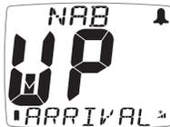
A waypoint arrival signal has been received from the GPS. The waypoint name is shown on the top line of the display.
