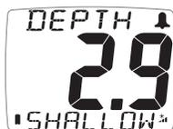
The water depth has fallen below the preset alarm level.
