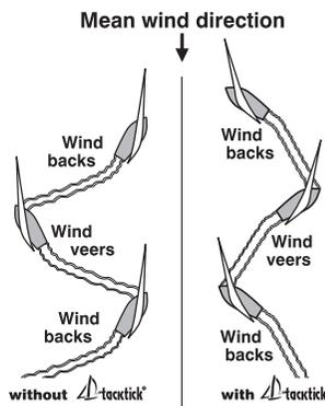
The system automatically calculates the mean wind direction by averaging the true wind direction over a period of time
