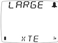
A large cross track error has been alerted by the GPS.
