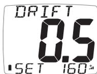
Because the boat is not always moving directly in the direction of its compass heading you need to know the direction (SET) and the speed (DRIFT) by which the boat is being pushed off course. Tactically this is important when assessing when to tack or gybe to round a mark or clear an obstruction or headland.
