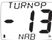
When steering towards a waypoint in tidal conditions, it is often difficult to assess the course to steer to keep on the direct track to the mark. Your Maxi Display automatically indicates when the course you are steering is taking you off the direct track to your waypoint. The direction and required angle of turn is displayed.
