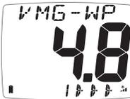
Use **VMG-WP** (VMG to Waypoint) together with the True Wind Angle to optimise your VMG to the downwind mark
