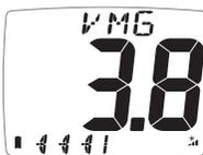
To get to the windward mark as quickly as possible it is necessary to balance pointing angle against boat speed to maximise the speed directly towards the wind (this speed is called the Velocity Made Good to Windward).
