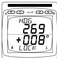
Heading locked at 269° now showing +008 change meaning current heading is 277°
