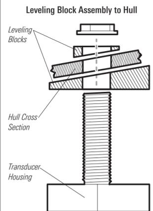
6. Apply a generous amount of marine-grade silicone sealant or slow-curing epoxy inside the drilled hole and along the mating surfaces of the transducer housing. Seal the mating edges of the leveling block (if using one) as well.
